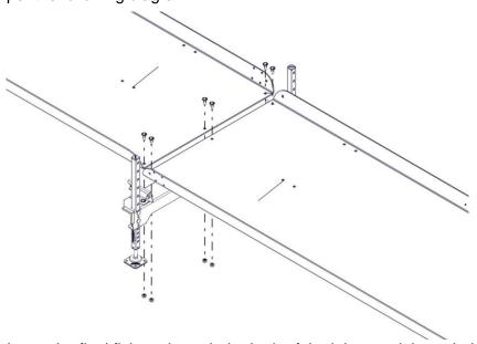
**6.** Insert the final fixings through the kerb of the joiner and through the kerb of the Permaramp:
